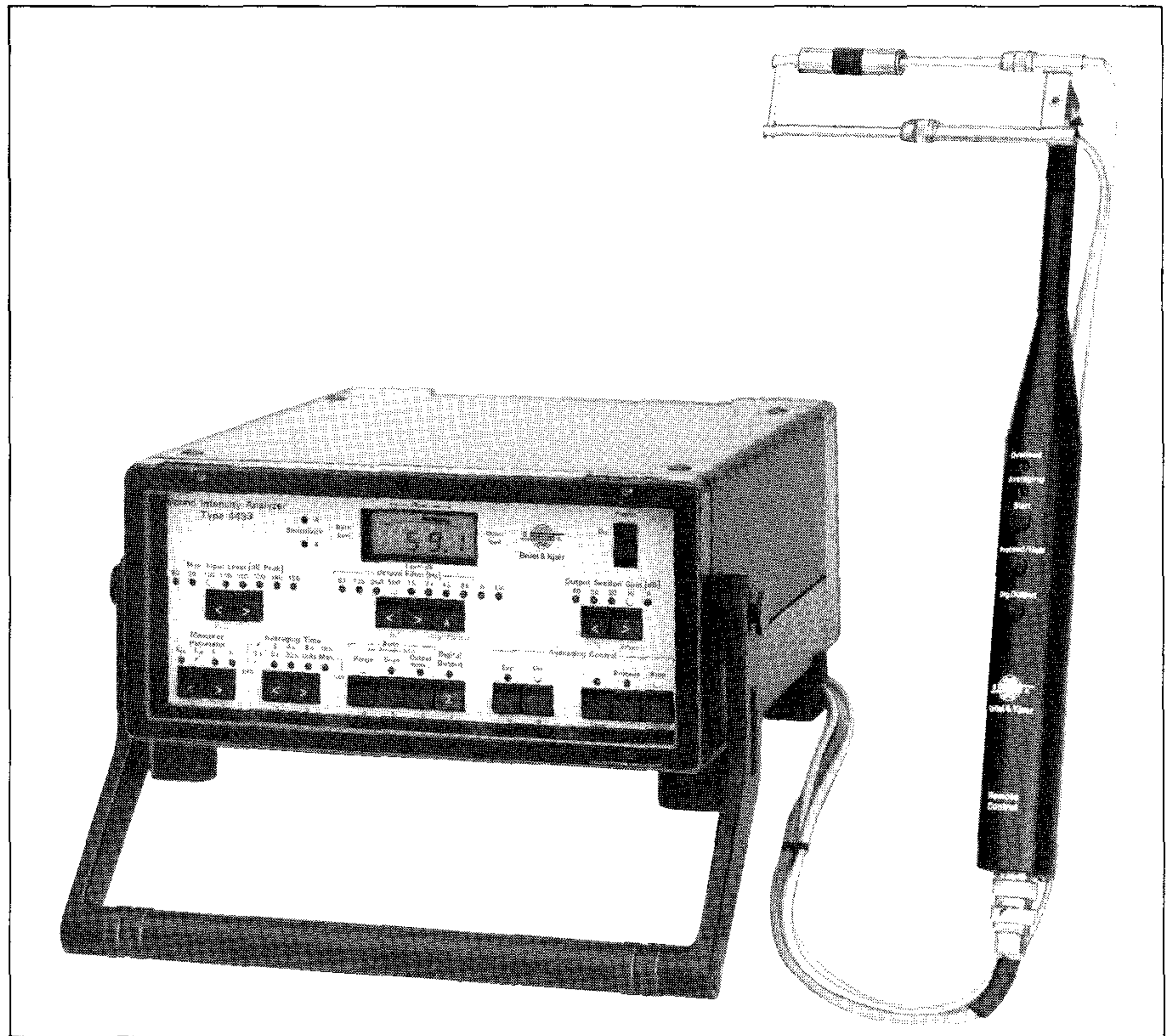
Fig. 4. Sound Intensity Analyzer Type 4433 and Probe Type 3520
